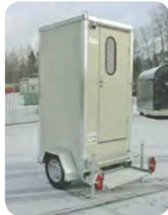
Toilet Wagon Tank Cabin mounted on chassis.
